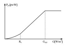
Fig. 3 Power model of the SCG
