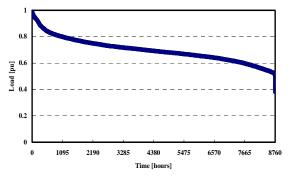
Fig. 9 Pattern of hourly peak load variation curve in the case
