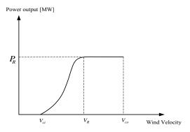
Fig. 1. Power output model of wind turbine generator
