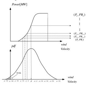
Fig. 2. Outage capacity *pdf* from the wind speed model combined the WTG power output model
