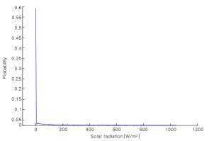
Fig. 10 Probabilistic distribution function of solar radiation at Jeju (1998~ 2007)
